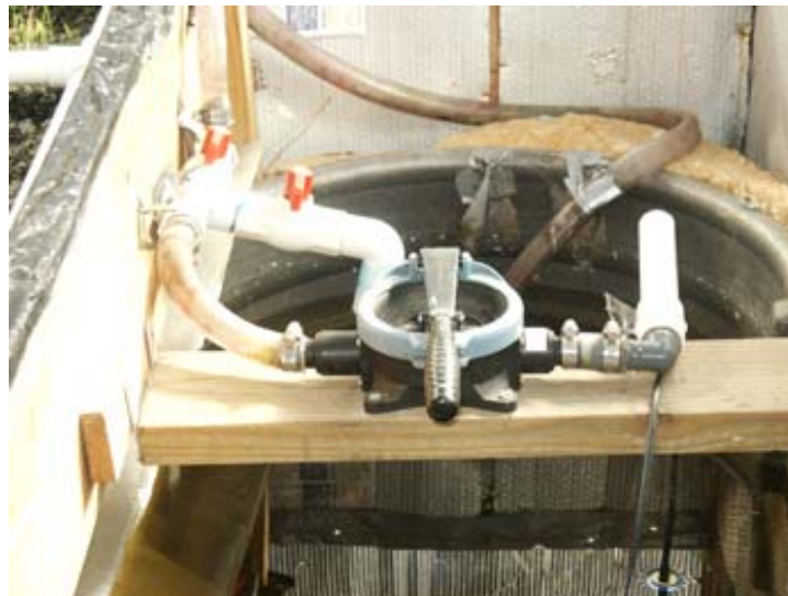
The manual pump assembly in the fish tank in the US prototype.
